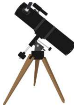
Figure (4) on the left. A refracting telescope with a smaller refracting telescope mounted on top as a guidescope. Figure (5) on the right. A reflecting telescope. Both scopes are on EQ mounts.
