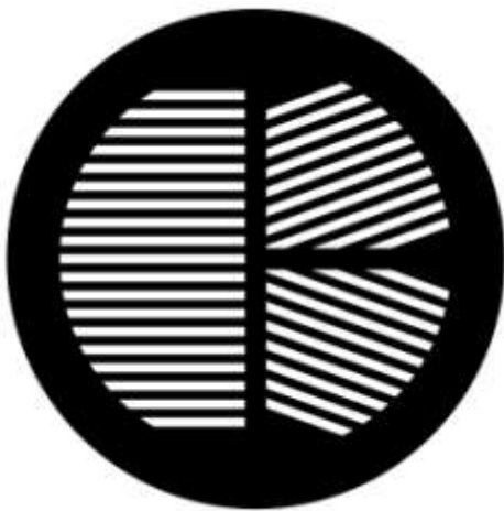
Figure (18). A typical Bahtinov Focusing Mask that fits over then end of the telescope.
