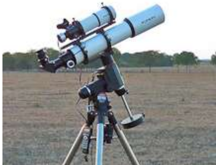
Figure (4) on the left. A refracting telescope with a smaller refracting telescope mounted on top as a guidescope. Figure (5) on the right. A reflecting telescope. Both scopes are on EQ mounts.
