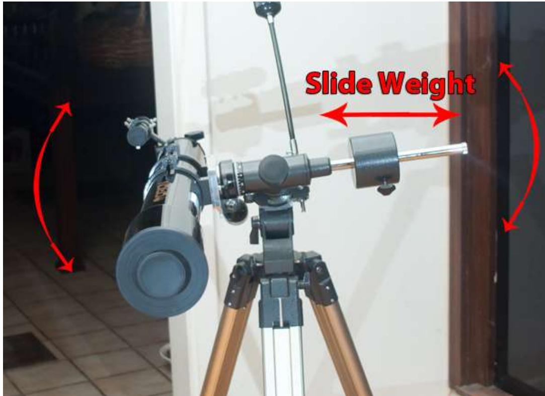
Figure (13). Balancing the scope tube.
