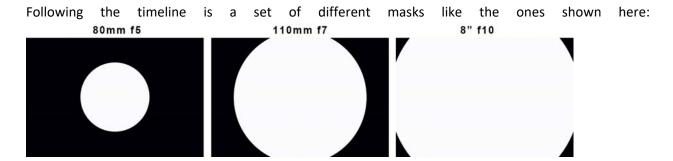
The three sections of the mask show the approximate size of a processed image relative to the size of an APS-C sized camera (crop sensor DSLR, also roughly the same as a 25mm 68 degree eyepiece field of view) in the telescope listed above each section.
