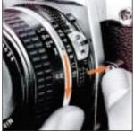
Lenses usable with the Nikon FA are Al-S Nikkor, Nikon Series E, Al-Nikkor, most Al-modified, and certain special lenses shown at the right. First line up the aperture/distance index 44 on the lens with the lens mounting index 15 on the camera body. Then twist the lens mounting ring 46 counterclockwise until the lens clicks into place Confirm that the aperture/distance index is exactly at the top.
