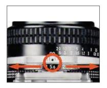
2. Set the lens to the desired fnumber. Although each number on the lens aperture ring has a click stop, you can also set the ring to intermediate settings. Note that small apertures give greater depth of feild, while large apertures restrict the zone of sharp focus to the main subject. The shutter speed dial can be set at any position except M250 and B
