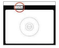
3. Check the LCD. Confirm that the LCD (liquid crystal display) is shown at the upper left in the viewfinder. This indicates that battery installation is correct and power is sufficient. If necessary, replace with a new set
