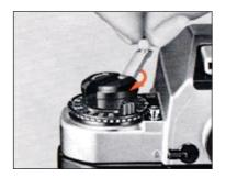
**3. Rewind the film** unfolding the film rewind crank and turning it in the direction of the arrow. When you feel the tension lessen, give it a few more turns until crank turns freely, indicating the film leader is rewound completely back into the cartridge.
