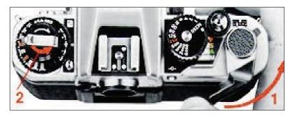
**7.** loading, continue to alternately ad vance the film and depress the shutter release button until the frame counter (7) reaches frame 1. While making blank exposures, check that the rewind knob is rotating, indicating the film has been loaded correctly and is being advanced. If the knob does not rotate, reload the film.
