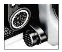
**4.** pattern metering is in operation by making sure that the metering control button is in the normal "out" position and the red index is not on top (refer to page 40 for more information)
