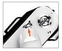
**2.** Depress the rewind button (3) on the bottom of the camera. You don't have to apply continuous pressure to the button; just press it once.
