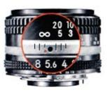
To create other-worldly effects, in which vegetation comes out light in tone and blue skies very dark, try shooting with black and-white infrared film In black and white infrared photography, you must use a red filter (R60) and refocus the lens to compensate for the fact that infrared light rays focus at a point slightly in front of visible Light For this purpose. most lenses have an infrared focusing index (47) (a red dot or line) beside the distance index (44) as a rule of thumb
