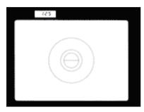
**4.** Look through the viewfinder and check the exposure **4.** information. Depress the shutter release button halfway and you will see the LCD showing the shutter speed (as a reciprocal) selected by the camera to provide correct exposure. Note that a slow shutter speed results in blurred images (techniques for avoiding blurred images are explained on page 46).
