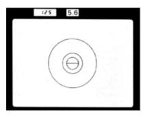
**4.** Look through the viewfinder and check the exposure information. The aperture you set is shown through the ADR window ①. When the shutter speed selected by the camera to obtain correct exposure with the aperture you set. If necessary, use a wider aperture to prevent a slow shutter speed from causing blurred images. (For additional information on avoiding blurred images, see page 46.)
