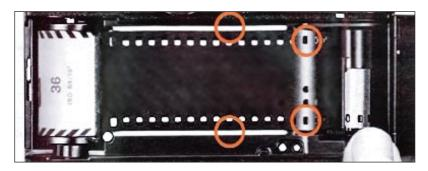
Advance the film by rotating the takeup spool further with your thumb. Make 2. sure the perforations on both film edges are securely engaged with the sprocket teeth. Also confirm that the film is properly seated between both film guide rails ⓐ and there is no film slack Then close the camera back until it snaps shut.
