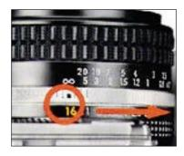
2. Set the lens to it's minimum aperture (the largest f-number). The shutter speed dial can be set at any position except M250 and B
