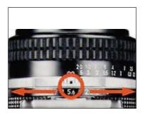
2. Set the lens to the desired fnumber. Although each number on the lens aperture ring has a click stop, you can also set the ring to intermediate settings.
