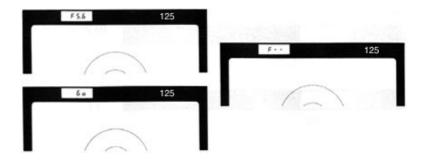
**5.** Look through the viewfinder and check the exposure information. The shutter speed you set is shown at The upper right-hand corner. When the shutter release button is depressed halfway, the LCD at the upper left-hand corner shows the aperture (a number preceded by F) selected by the camera to match the shutter speed you selected
