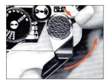
A multiple exposure is created by taking more than one shot on the same frame of film. Follow this procedure:
