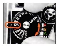
**3.** the shutter speed dial to the desired shutter speed. The numbers on the dial are reciprocals, e.g., 4000 means 1/4000sec. The 250 engraved in red indicates the fastest sync speed for an electronic flash unit. Each setting has a click stop.
