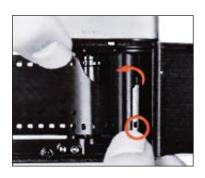
4. with the sprocket teeth. Turn the takeup spool slightly with your thumb, so that the first or second perforation at the bottom edge of the film s engaged with the small tooth at the bottom of the slot in the takeout spool, and the top and bottom perforations mesh securely with the sprockets (35)
