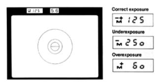
**4. Center your main subject in the viewfinder and check 4. the exposure information.** Remember that in the manual mode, centerweighted metering is always in operation regardless of the position of the metering control button. The selected f-number is shown through the ADR window When the shutter release button is depressed halfway, the LCD shows the selected shutter speed preceded by the letter M.
